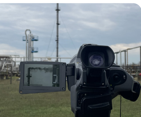
Figure 1: CATF’s Methane Pollution Prevention team has surveyed over 500 oil and gas sites around Europe for methane leaks, finding evidence of emissions in 342 (Credits: Mihai Stoica).
