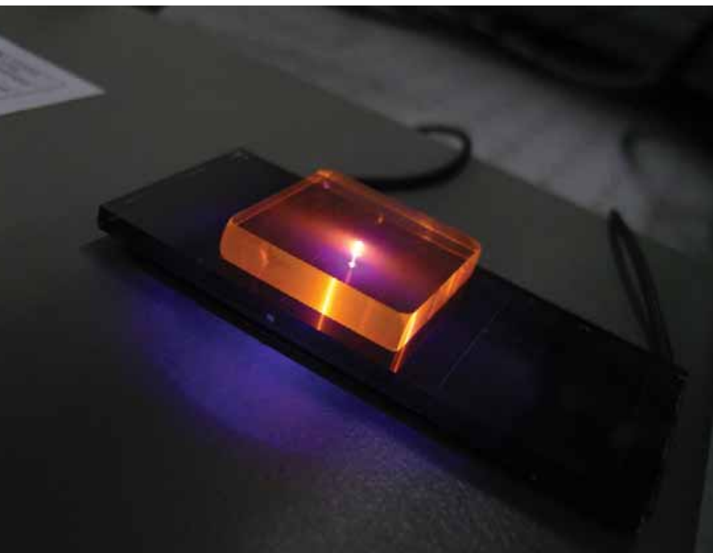
Figure 1: Samarium-doped glass on a CdTe thin film solar cell under UV excitation.
